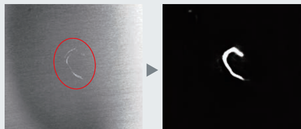
White scratch on shaded hairline finish
