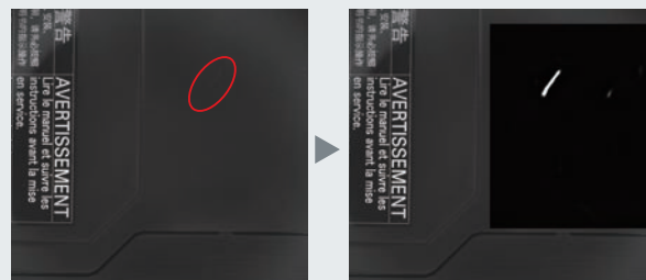
Scratch on resin products
