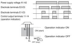
When the liquid level reaches E1 (indicator turns ON), the pump starts.
