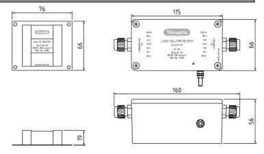
Figure 2: Dimensions of the load cell protectors
