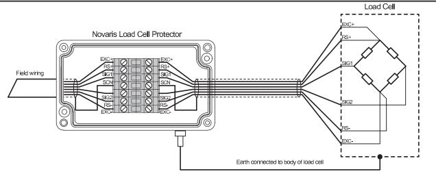
Figure 3: Installation of load cell protector
