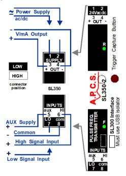
Terminals 1 to 2 power the unit with 2.5kVrms galvanic isolation to other terminals. Check labelling at the terminals for correct supply voltage.
