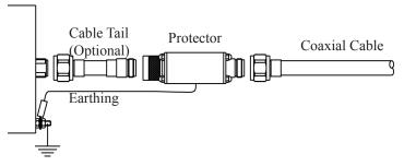
Figure 3: Connection of Novaris Coaxial CCTV Protec-
