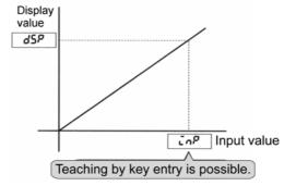
To allow a readout of 10.000 when the input value is 4.2 kHz (= 4200 Hz), for example, set the parameters as follows.
