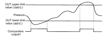
• When the internal temperature reaches 1000  $^{\circ}$ C or lower than 800  $^{\circ}$ C, comparative output 1 is turned ON.
