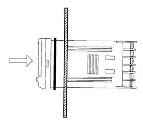
(3) Put the adapter in the fixing grooves on the left and right surfaces of the rear case, push it until it contacts with the panel, and fix it.
