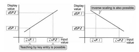
Inverse scaling where readout decreases with increasing input is also possible.
